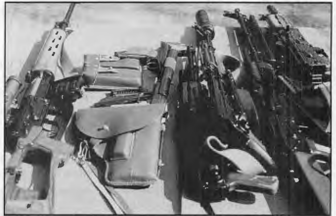
Toys for big boys: from left is scoped Dragunov sniper rifle, standard Makarov pistols, suppressed PB-69 Makarov, two folding-stock AKs, one of which has a suppressor, late model RPK-74 light machine gun, AKSU-74 submachine gun.
